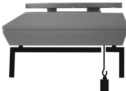
Fig. 1: Setup of balance for underfloor weighing
